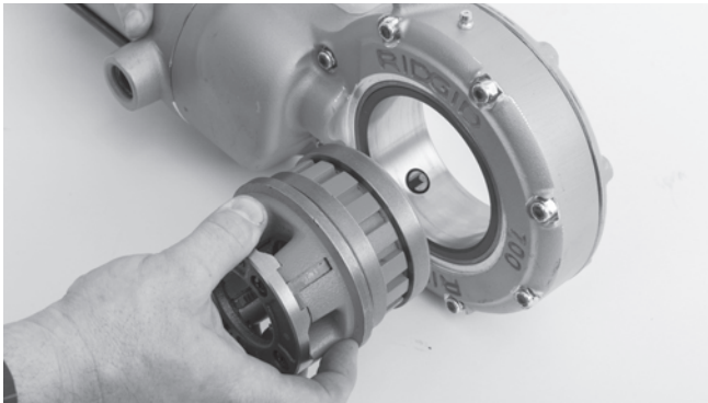
Figure 4 – Installing Die Heads into 700 Power Drive
