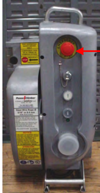
Emergency Stop Button
