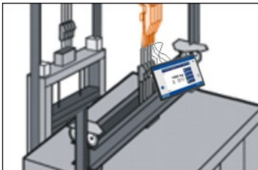
Illustration 99: Positioning of MSM12 and Sensors for 1:1 Suspension
