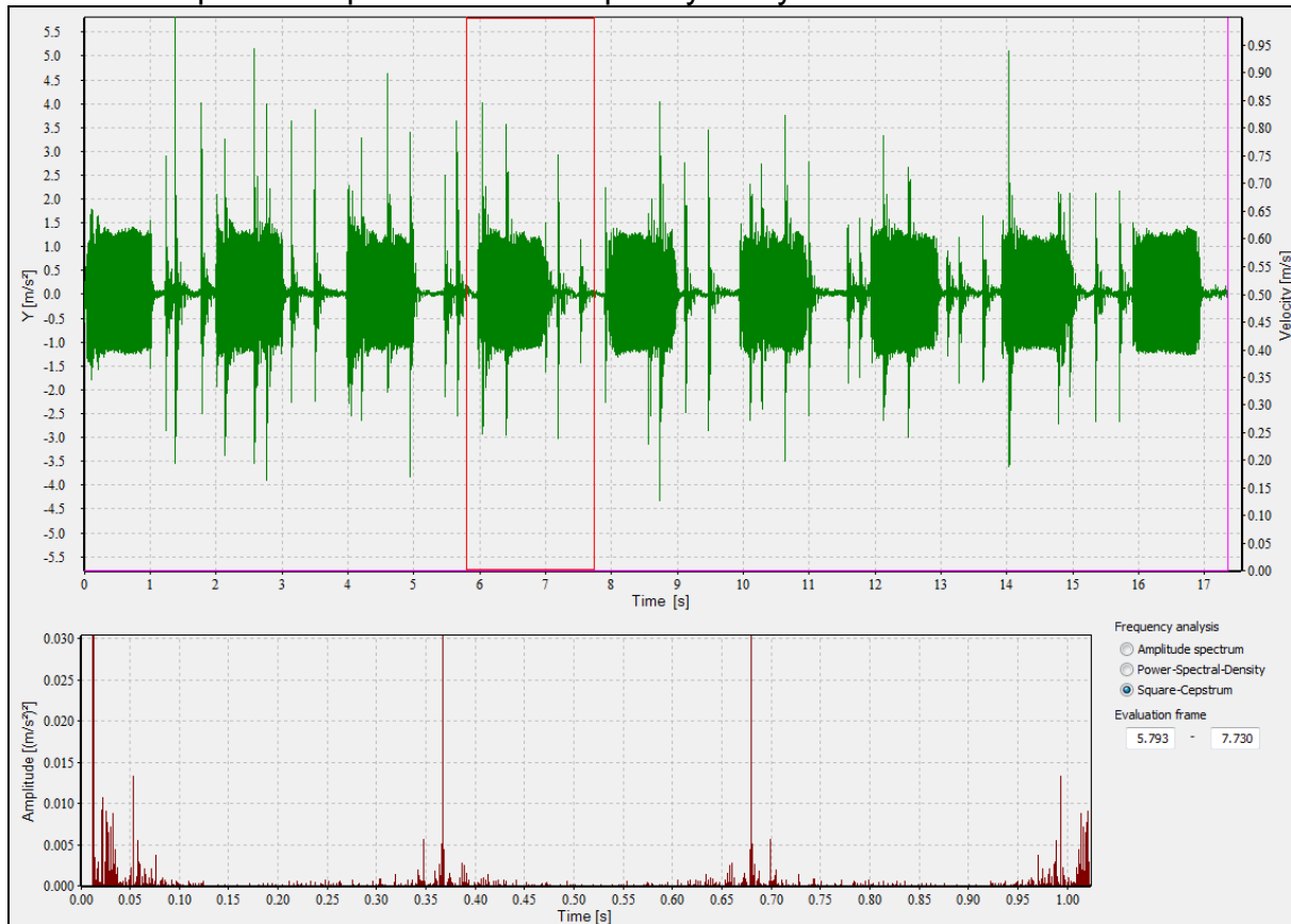
Illustration 63: Display of the square Cepstrum in the lower third of the screenshot
