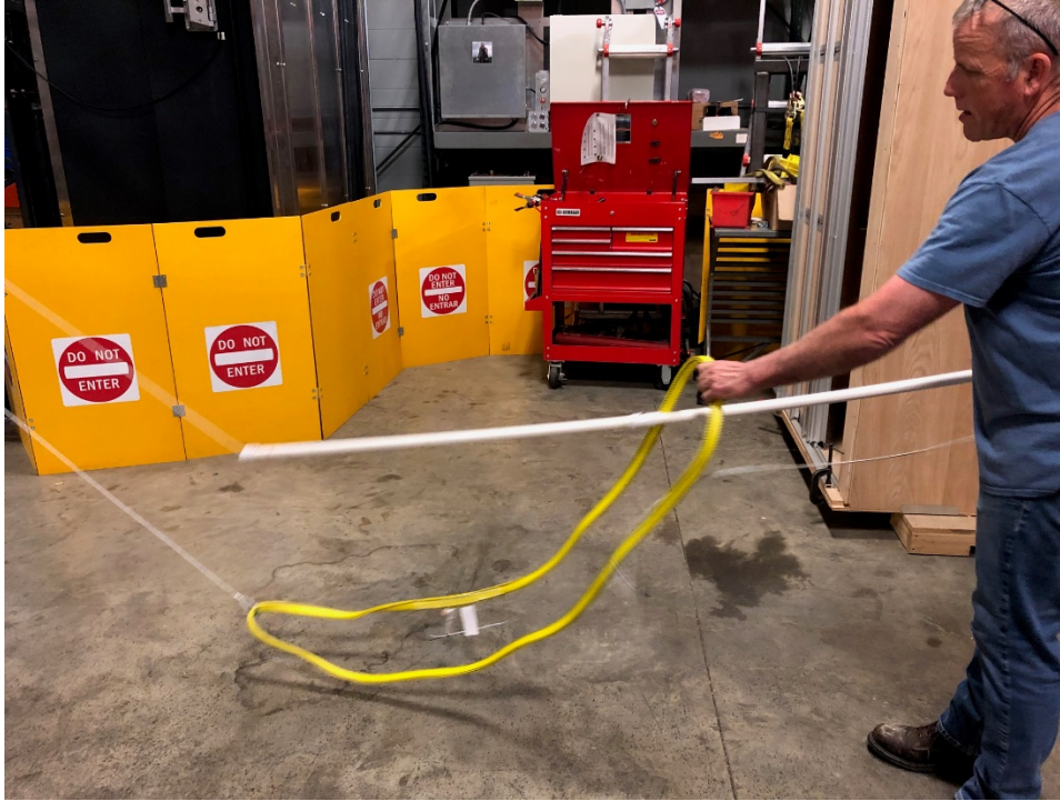
Step 5: Cinch the nylon web sling back up and over the beam.
