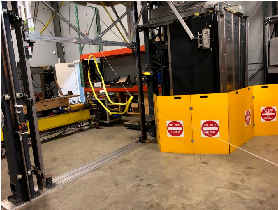
Step 5: Cinch the nylon web sling back up and over the beam.
