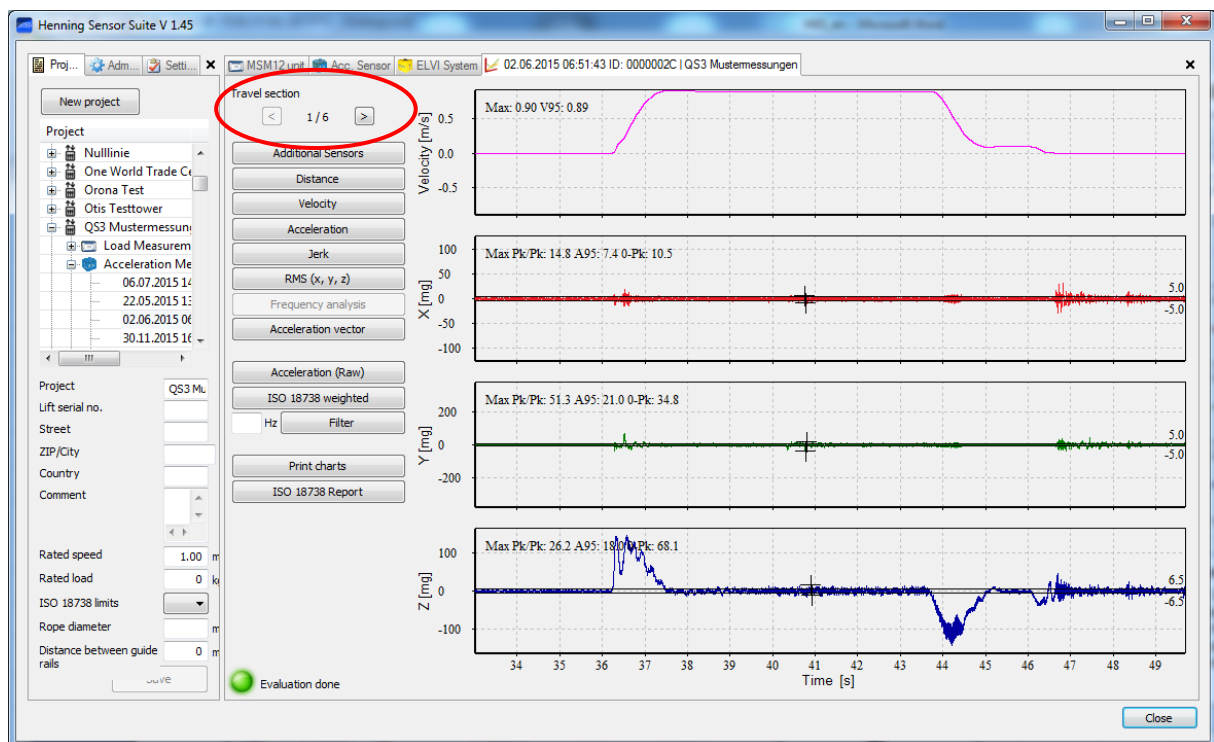
Figure 48: Curve representation of an acceleration measurement
