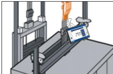
Illustration 99: Positioning of MSM12 and Sensors for 1:1 Suspension
